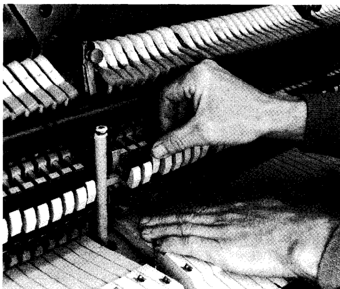
Photo 4: Check wippen flanges by depressing soft and sustain pedals, holding back ends of keys down, lifting wippens part way and dropping back onto capstans
