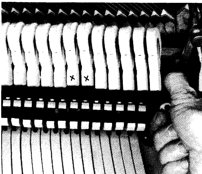
Photo 3: Pull back on hammer rail for a quick check of lost motion—the two hammers marked X stand off the rail, showing no lost motion
