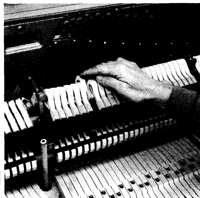
Photo 2: Lift individual hammers halfway to strings and release, watching for fast return and a slight bounce off rail
