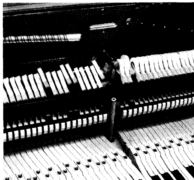
Photo 1: Press and release soft pedal quickly as a quick check for sluggish hammer return
